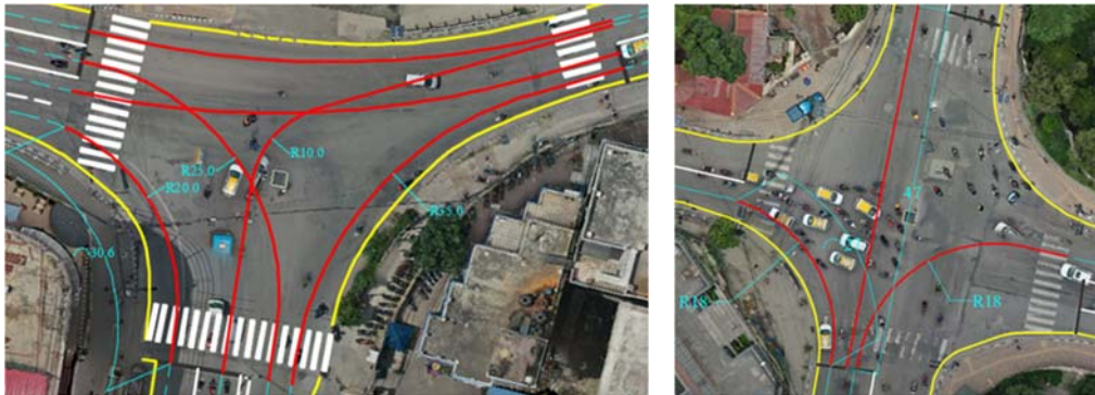
Figure 3: Sample of Negotiation Distance and Radius Measurement
