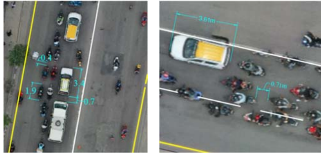
Figure 2: Sample for measurement of Queue Space and Vehicle Length
